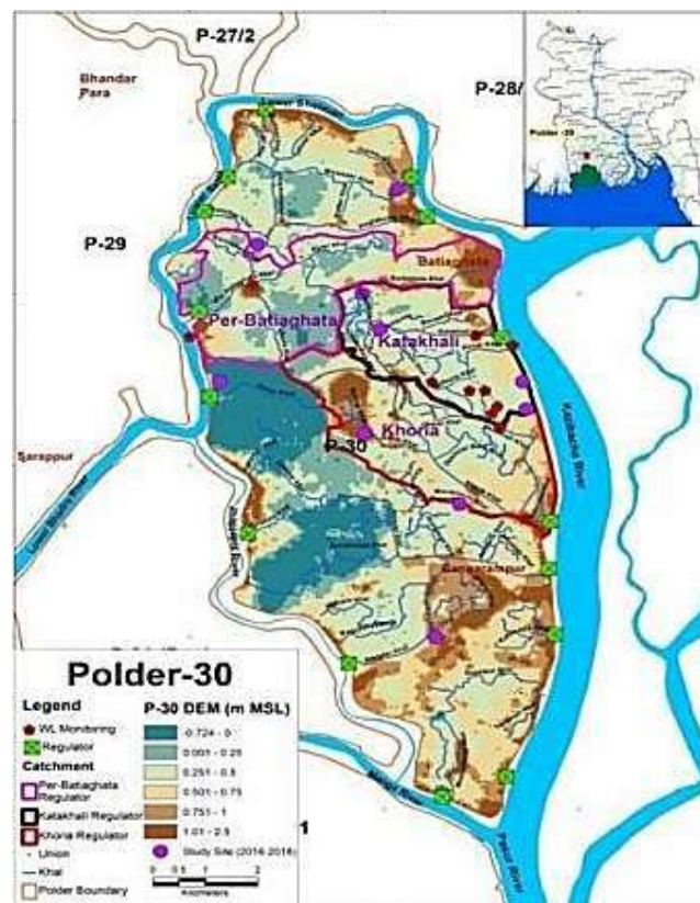
Figure 10. Map of Polder 30 showing the basin areas of the regulators and study sites (Mondal et al. , 2019)
