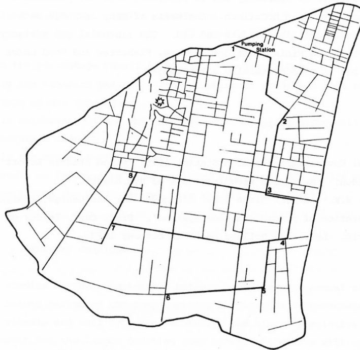
Figure 12. Drainage network of the Newborough Fen with location of water level recorders (Beran, 1983)
