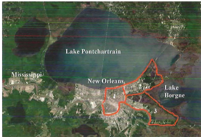
Figure 5. Polders (red encircled) – Orleans (1), Orleans East (2) and St. Bernard (3) - in New Orleans that were flooded due to the hurricane Katrina in 2005 (Kok et al., 2006)
